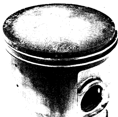
20:1 Our baseline premix ratio produced 26.9 bhp and the light coating of piston varnish seen here.
